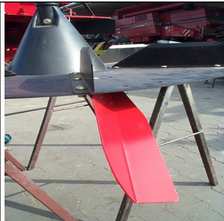
photo showing right disc of AF 1680/2188/2388 with diagonally cutted upper wings and lower windwings.
